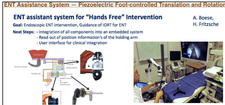
Piezoelectric driven endoscopic holder for ENT applications
